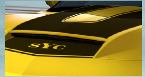
RTM hood with integrated scoop; Yenko sYc® hood stripes; GM heritage-style front grille with body color painted surround.
